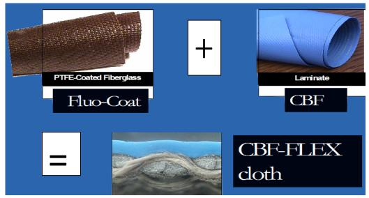
The harsh environment faced by expansion joints in Flue Gas Duct include: corrosive flow medium, temperature fluctuation from high to low and the condensation, mechanical stress by duct movements. Many joints made of PTFE coated and or film laminated fiberglass with low PTFE content or weak film strength failed unexpectedly causing tremendous loss.
